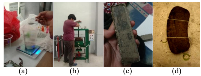
Fig 1. making samples (a) weighing materials (b) compaction process (c) brake lining (d) formed brake lining
