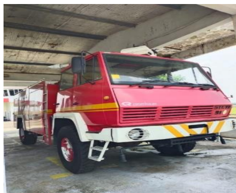
Gambar 4. Foam Tender Type IV (Roseunbauer)
