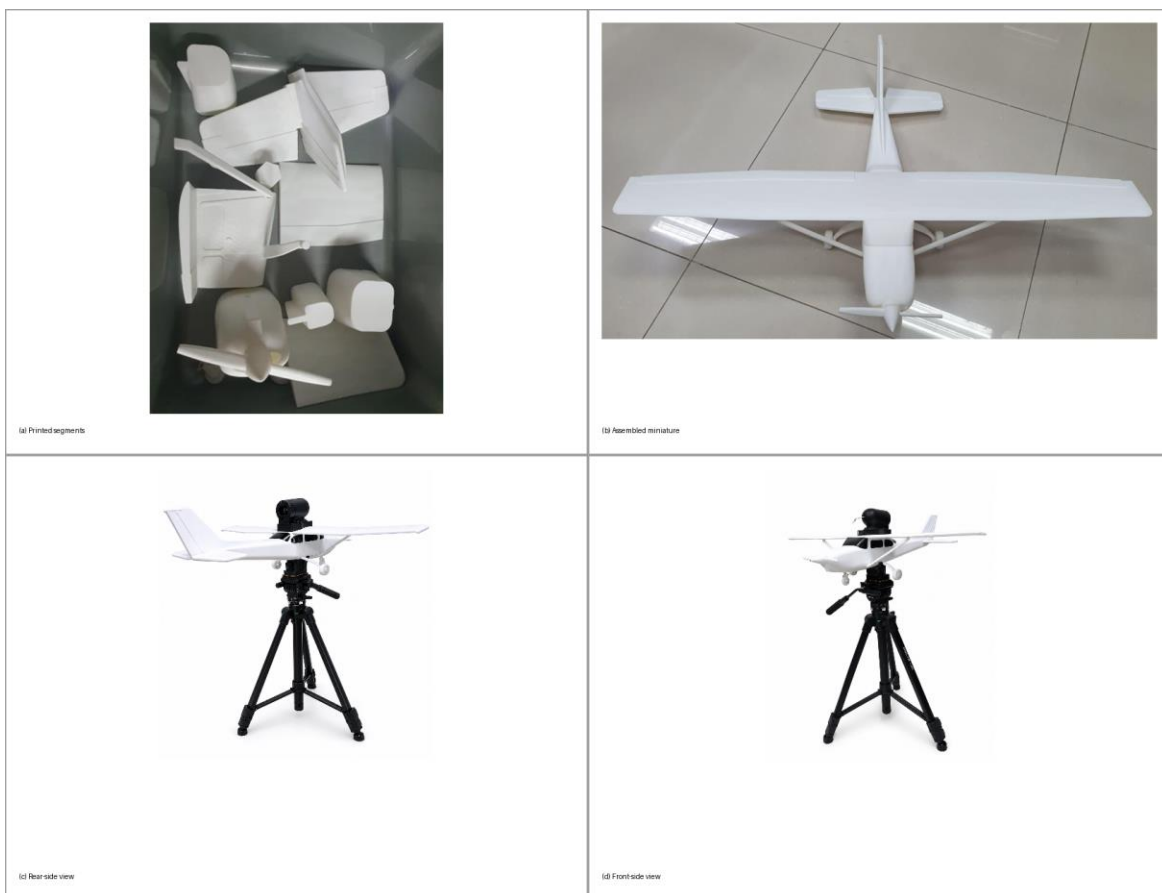
Figure 3. Fabrication and assembly stages showing segmented printed airframe components, the assembled airframe, external compass installation, and the final tripod-mounted trainer configuration
